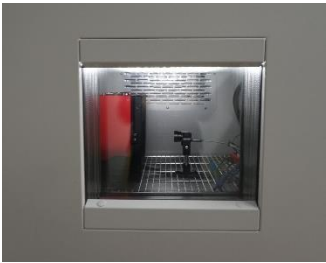
IR camera being tested in Piséo's climate chamber
